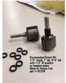
8. Use Router with suggested bit to rout cavity along front, back and sides of Pocket Rout template. I use Two templates to set the depth of the router. 0.44". When locked at that depth, and using the pocket rout template on the guitar, it leaves the original shape of your cavity as it was, and starts the rout 0.22" below the back of the guitar.
